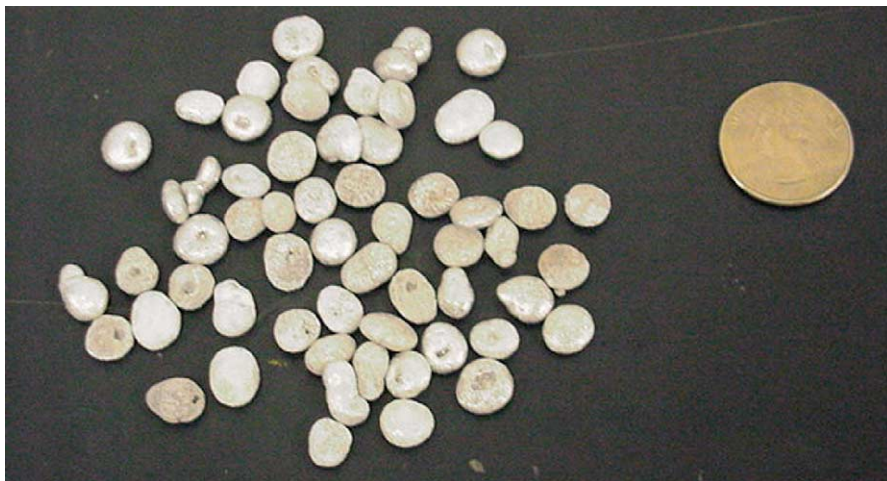
Fig. 2. Granular aluminum anode, 8–12 mm in diameter, 99.9% purity.
